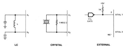
ALTERNATE FREQUENCY REFERENCE OPTIONS (COMPONENT VALUES TO BE DETERMINED)
